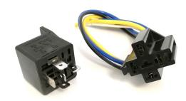
Pumps should be supplied power through a relay that provides power directly from 12v source. Use a fan switch or manual switch to trigger the relay. Harness/plug is included, 12 volt 30/40 amp rated.
