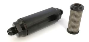
Most in-line filters are not specifically designed to work in circulation/cooling applications; fuel filters are far too restrictive and drysump screen elements can let through particles that can jam gears and tear soft parts (diaphragms). Our specially designed in-line oil filter protects oil pumps circulation from foreign object damage by filtering particles down to 240 micron without restricting oil flow.
